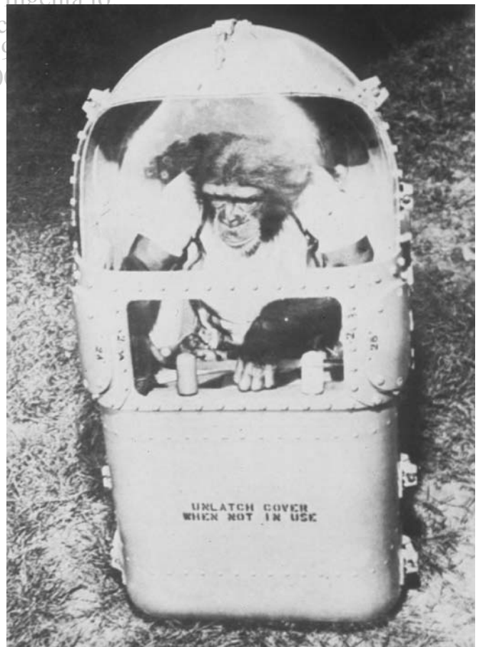
Fig. 5. Insulated flight couch and work panel for animal pretest flights of Project Mercury. Personal collection of the author.
